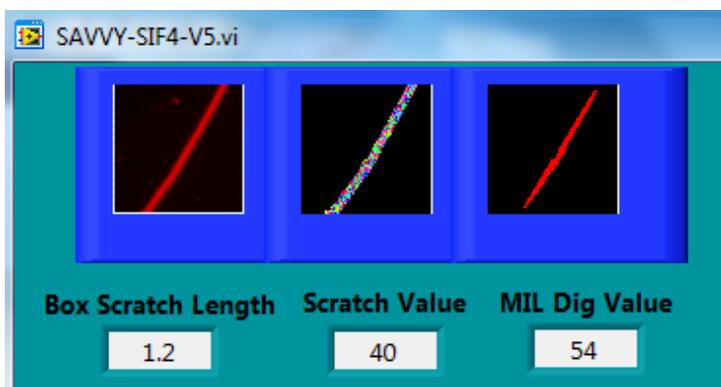
Figure 6. Upper left corner of SavvyInspector™ window during a scratch inspection.
