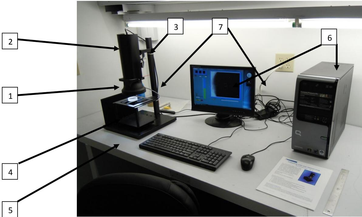
Figure 1. Typical SIF-4 installation.
