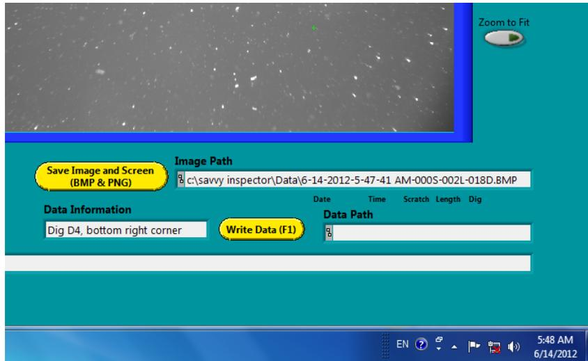
Figure 8. Pressing the “Save Image and Screen” button stores the screen shot and image data into the image path noted at the right.
