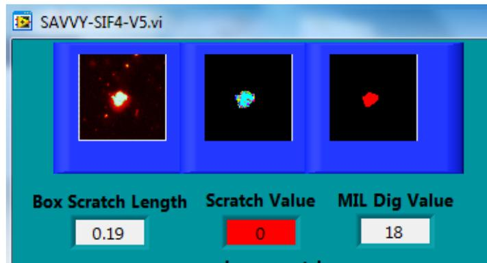
Figure 10. Upper left corner of SavvyInspector™ window during a dig inspection.
