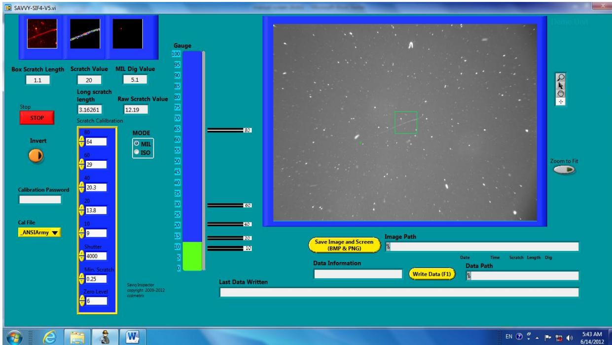
Figure 7. When the stage is translated, the Long scratch length box reports the total motion of the stage. When the ends of the scratch are used for the start and end of the translation, the result is the length of the scratch; in this case 3.16mm.
