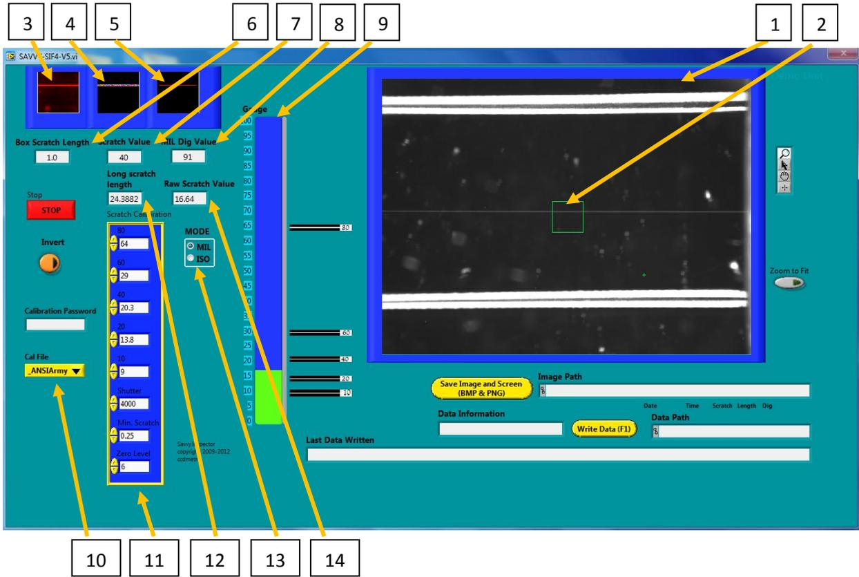
Figure 2a and 2b. Diagram of the Inspection Software Features
