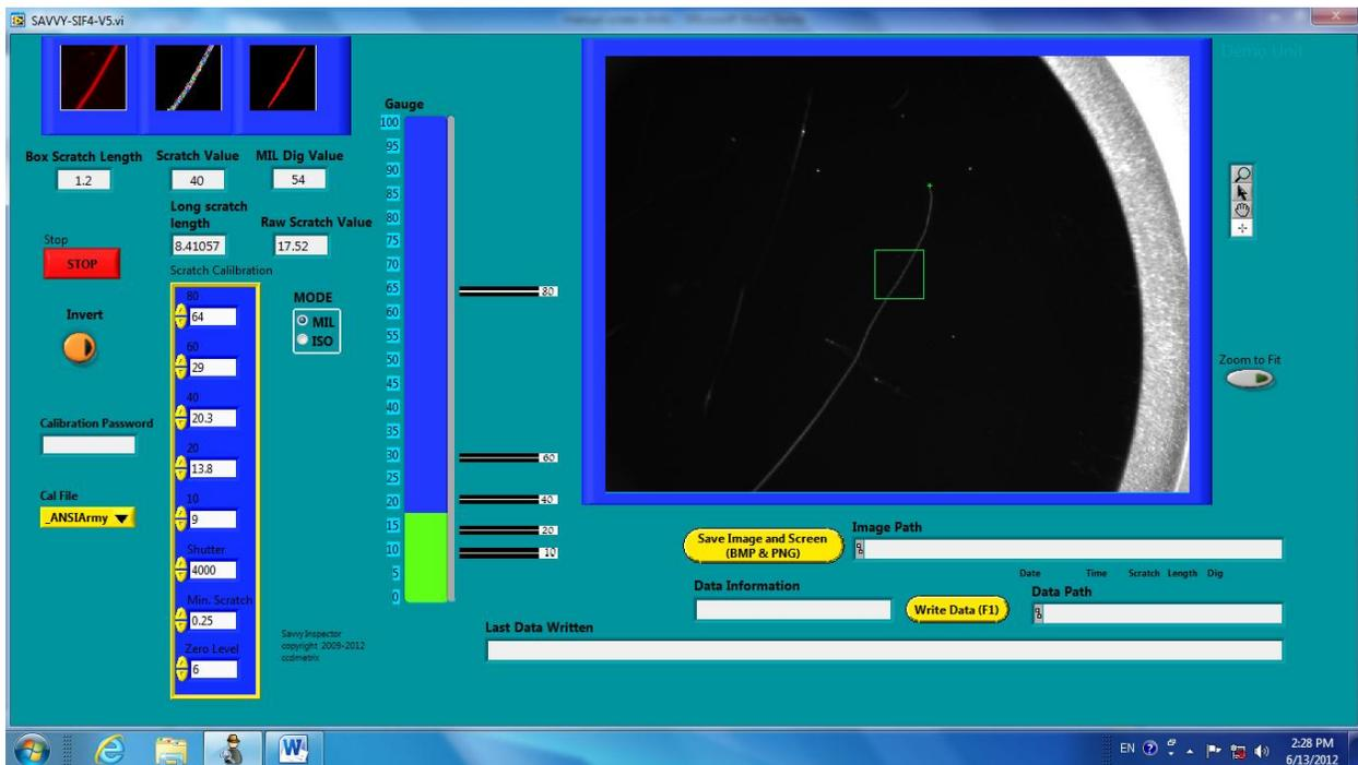
Figure 5. The SavvyInspector™ window during a scratch inspection.
